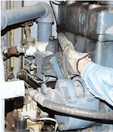
9. Open the compression release valve by pulling the handle toward you
