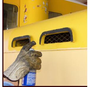
10. Spray (about one second) starter fluid into each of the two intake vents
