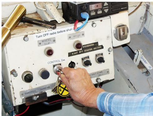
2. Using the key, turn on the CONTROL switch
