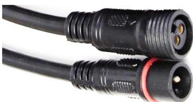
The connectors tentatively selected are pre-molded two-pin waterproof IP65, are AWG18, and are used for outdoor LED wiring. They come with a 8" cable stub, so must then be spliced into the overall cable system. These connectors do have a securing (threaded nut type) ring available, but it doesn't need to be used.
